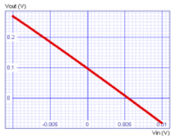
Figure 11: DC Voltage Offset of Inverter
