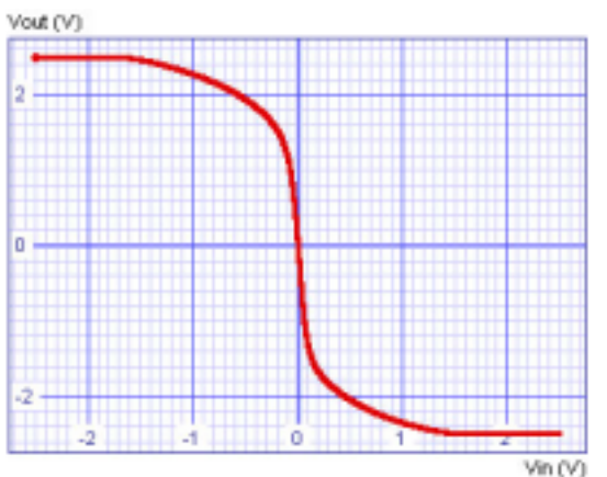
Figure 10: Transfer Characteristic of Inverter
